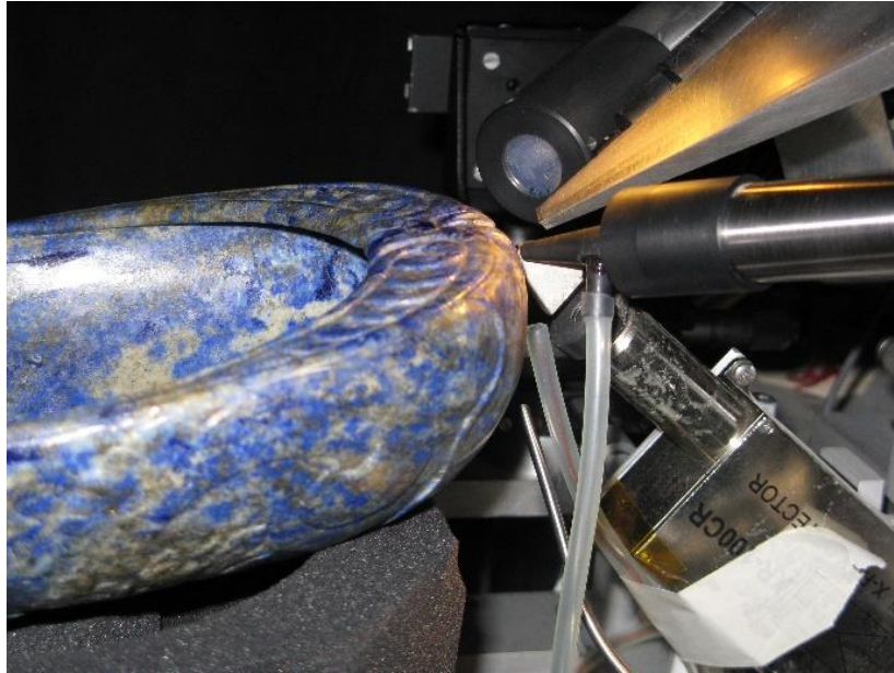
Figure 3 - Experimental set-up of the external microbeam line at INFN-LABEC in Firenze during the analysis of the Oval Bowl (“Collezione Medicea”).
