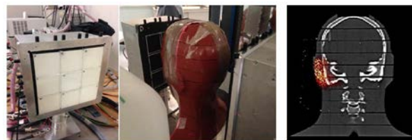
Left: one head of the DoPET prototype. Center: the prototype ready for the data taking with an anthropomorphic phantom at CNAO, Pavia, Italy. Right: a slice of the reconstructed activity after a 2Gy proton treatment plan.
