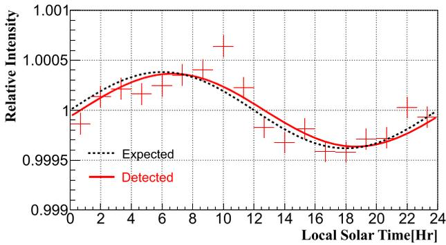
**Figure 6.** Projection of the event distribution in solar time for  $N_{\text{hits}} > 500$ . The dotted line represents the expected Compton–Getting modulation. The abscissa bars present the width of bins and the ordinate errors are statistical.
