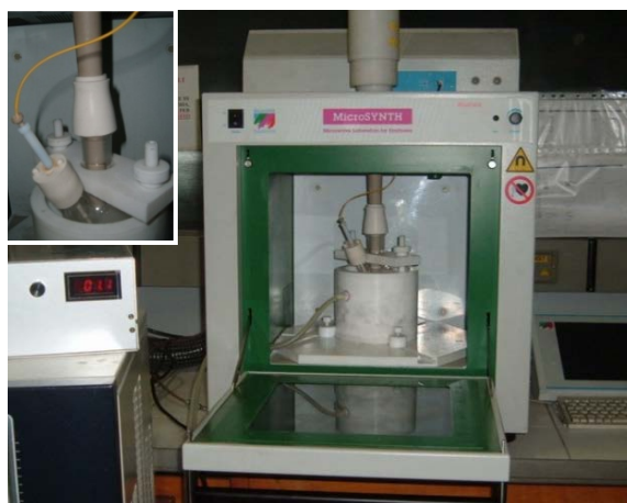
Figure 4. SMUI with a cooling system (Authors' lab)
