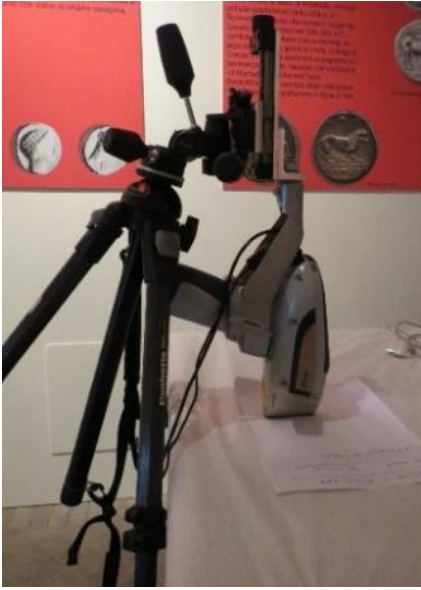
Fig. 2. p-XRF setup during measuring session in museum.
