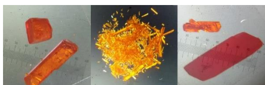
Figure 2 . Single crystals of compounds 1 (left), 2 (middle) and 3solv,(right) obtained by recrystallization from solution of the mechanochemical synthesis products (see Experimental).
