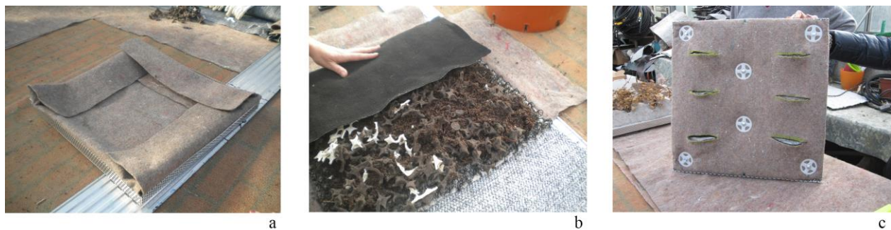
Fig. 2. Manufacturing of the final prototype. Fig. 2a) Outer layer of the VGMS (recycled polypropylene). Fig. 2b) Placement of the inner layer (growing medium) of the VGMS. Fig. 2c) Modular box of the VGMS with pockets where the plants were to be inserted.
