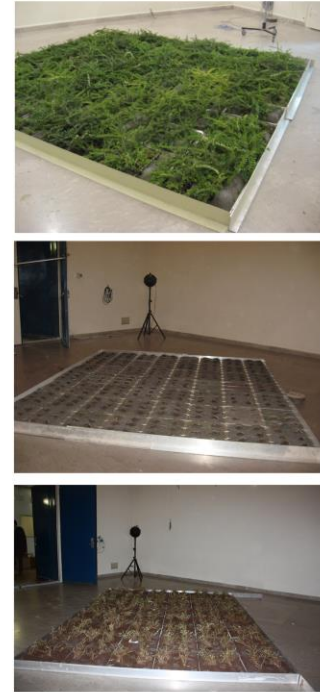
Fig. 15. Experimental sound absorption coefficient results in the reverberation room. The three different prototypes measured in the reverberation room were: VGMS_1, VGMS_1 without plants and soil, VGMS_2 (c).
