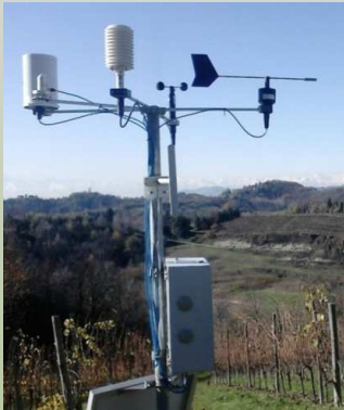
Fig. 1 – VA Automatic Weather Station in conformity with WMO recommendations
