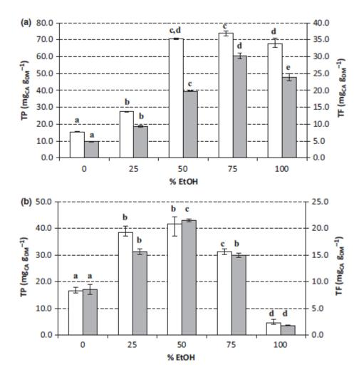
Fig. 1. TP yields ( $\square$ ) expressed as  $mg_{GAE}/g_{DM}$ , and TF yields ( $\square$ ), expressed as  $mg_{CE}/g_{DM}$ , of Croatina GM extracts using HPTE (a) and UAE (b) techniques with different ethanol/water ratio solvents. Different letters indicate significant differences in data at p < 0.05.
