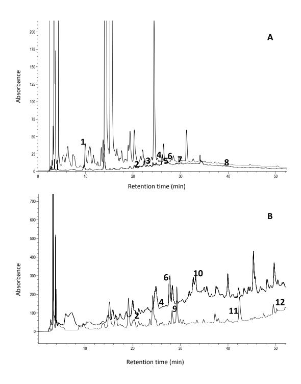
**Fig. 3.** HPLC chromatograms of grape marc (A) and olive pomace (B) extracts using UAE (dashed lines) and HPTE (continuous lines) with 75:25 ethanol/water.
