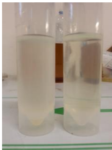
Figure 3. Rapid test on biodiesel (unwashed) from palm oil. Left: sample after the 1 st step of reaction. Right: after the 2 nd step of the reaction.
