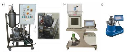
Figure 1. a) Rotor-stator generator of hydrodynamic cavitation \_E-PIC S.r.l. (Turin, Italy). b) The configuration of FlowSynth Microwave system (Milestone S.r.l.). c) High-Shear Mixing (Magic-Lab, IKA).
