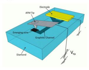
Fig. 2: Schematics of the experimental set-up. The AFM tip is scanned on the emerging end-zone of the graphitic channel. The electrostatic potential on AFM tip is set to a positive value and the current flowing through the tip, the graphitic channel and the electrode is measured for every point of the scan.
