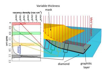
Fig. 1: Schematics of the implantation through a variable-thickness mask (right) and corresponding SRIM evaluation of vacancy density profiles generated in diamond at variable depth by 1.2 MeV He<sup>+</sup> irradiation after crossing the copper mask
