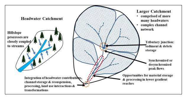
**Figure 15.** Comparison of processes affecting the movement of water, sediment, nutrients, and contaminants from upstream to downstream reaches, as influenced by the channel network characteristics. Based on the concept introduced by Gomi et al. (2002).
