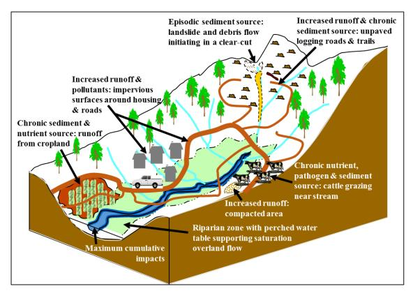
**Figure 14.** An example of how land uses within a catchment can generate cumulative effects related to streamflow regime, sedimentation, and nutrient/pollutant fate and transport.
