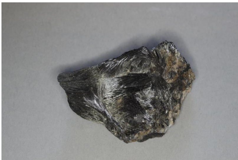
Figure 13. " Speziaite ". Sample of ferro-ferri-hornblende, described by Colomba in 1914 and dedicated to Ing. Giorgio Spezia as "speziaite". The mineral was later discredited, and was redefined by Oberti et al. (2016). The sample, six-centimeter-long, belong to the collection of the Regional Museum of Natural Science, Torino, catalog number MU15285.
