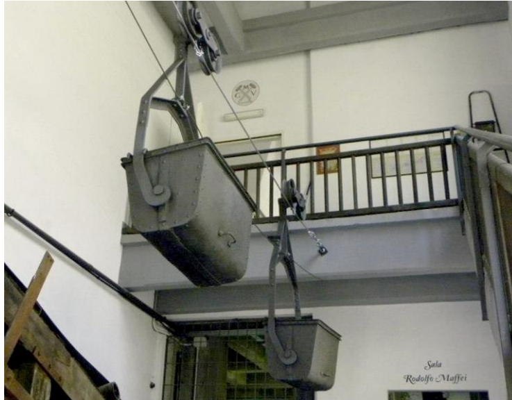
Figure 15. Two old suspended carts used for the transportation of ore from the mine to the crushing and milling area, now at the main entrance of the Museum of Traversella.
