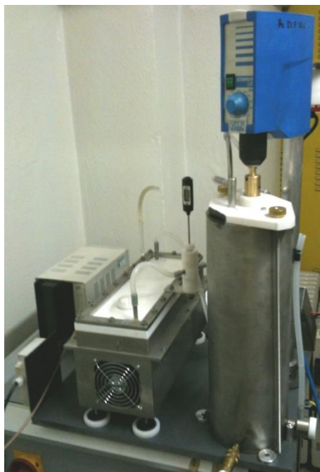
Figure 5. Complete view of the flow reactor with tank, thermometer and mechanical stirrer on the right. The flow reactor operates in the following manner (Fig. 6):
