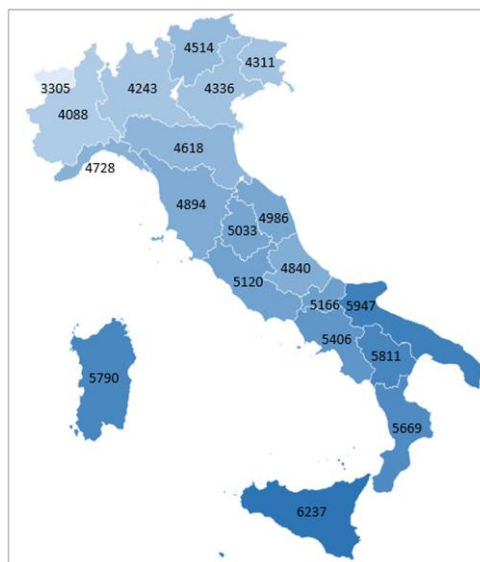
Figure 2. Average values for the different Italian Regions of CWR based on maize crop cultivation ( \text{m}^3 \text{ha}^{-1} ).
