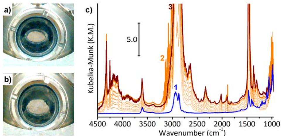
MgCl<sub>2-250</sub>/TiCl<sub>4-90</sub>/TEA catalyst (from spectrum 1 to spectrum 2) and after flushing the cell with pure N<sub>2</sub> flux (spectrum 3). The spectra upon ethylene polymerization were collected every minute for 10 minutes.
