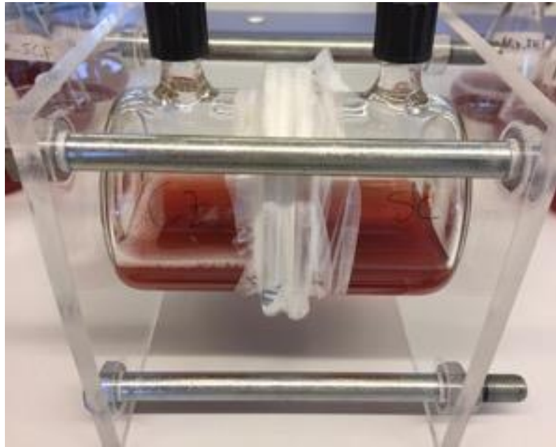
Figure S1. Double-compartment fermentation system consisted of two glass chambers with loose screw cap, separated by a 0.45 \mu\text{m} membrane filter. The filter membrane allows the exchange of metabolites keeping separated cells belonging to two different species.
