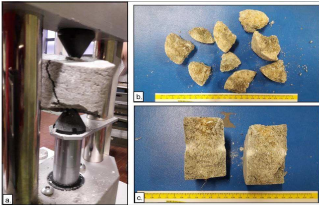
Fig. 7. (a) Macroscopic observations of sample failure during PLTs; (b) Post-failure rock fragments of samples with I_{50} values lower than 0.5-0.6 MPa; and (c) Post-failure rock fragments of samples with I_{50} values higher than 0.5-0.6 MPa.
