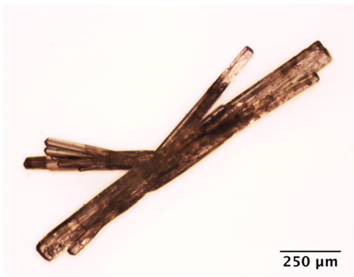
Figure 12 – Optical micrograph of \text{Ce}_2(\text{NDC})_3(\text{DMF})_2 crystals.
