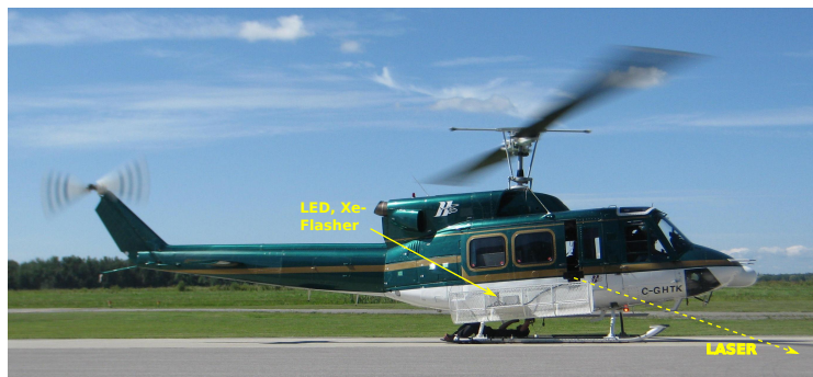
Figure 3: The light sources were mounted on a Bell 212 helicopter. This dual turbine model was used because it satisfied various rules for night flight in Canada.
