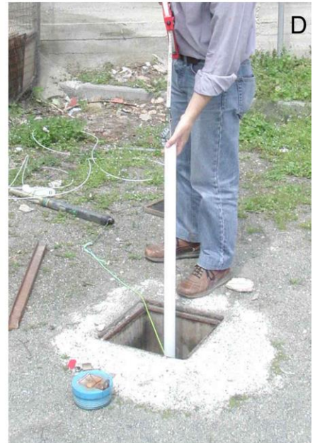
Fig. 4. Multilevel sampling devices used in the Racconigi piezometer. A) multiprobe meter for multiparameter logging. B) packer system. C) dialysis membrane sampler. D) bailer.
