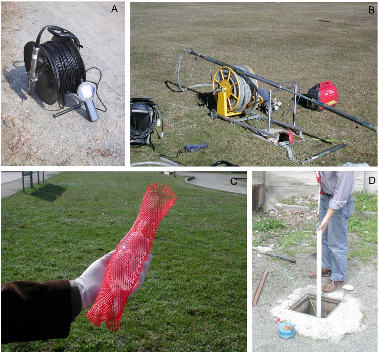
Fig. 4. Multilevel sampling devices used in the Racconigi piezometer. A) multiprobe meter for multiparameter logging. B) packer system. C) dialysis membrane sampler. D) bailer.
