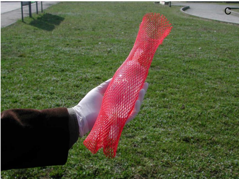
Fig. 4. Multilevel sampling devices used in the Racconigi piezometer. A) multiprobe meter for multiparameter logging. B) packer system. C) dialysis membrane sampler. D) bailer.
