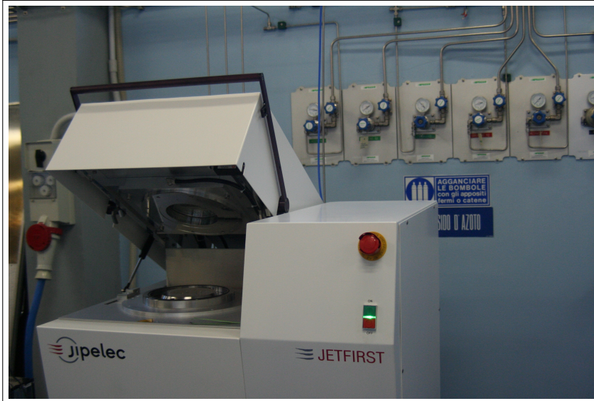
Figure 73: RTA system for CVD processes at I.N.Ri.M.. Picture of the system for graphene synthesis present at I.N.Ri.M. laboratories. The system is equipped with four gas lines and allows for fast cooling, being a cold-wall system: flash graphene growth processes can be therefore tested.
