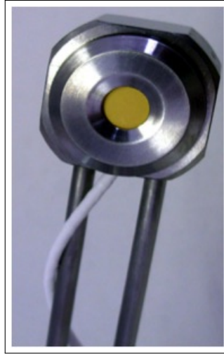
Figure 42: Quartz Crystal Microbalance for thickness detection. Head of the crystal sensor placed inside the thermal and e-beam evaporators at I.N.Ri.M. for real-time detection of the film thickness and growth rate during thin film deposition processes.
