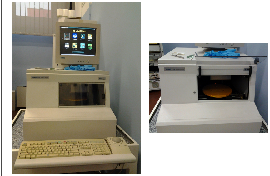
Figure 41: Profilometre at I.N.Ri.M.. Picture of the profilometre used at I.N.Ri.M. to determine the roughness and the thickness of thin films.
