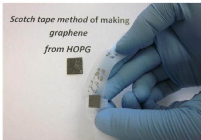
Figure 30: Mechanical exfoliation of graphene. Image showing the mechanical exfoliation procedure employed to deposit monolayer graphene from HOPG by means of a scotch tape. The technique allows to obtain high quality graphene, but it is not scalable. Adapted from [165].
