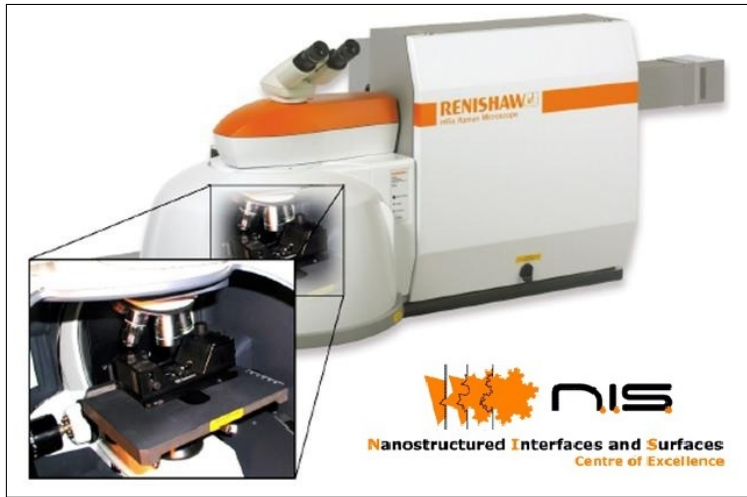
Figure 103: Instrumentation for Raman spectroscopy at NIS Centre - Turin. Image of the Raman spectrometer present at NIS Centre - Turin employed for graphene characterization. The instrument is equipped with four laser exciting lines, but I have always worked at only two wavelengths: 442 nm and 514 nm.
