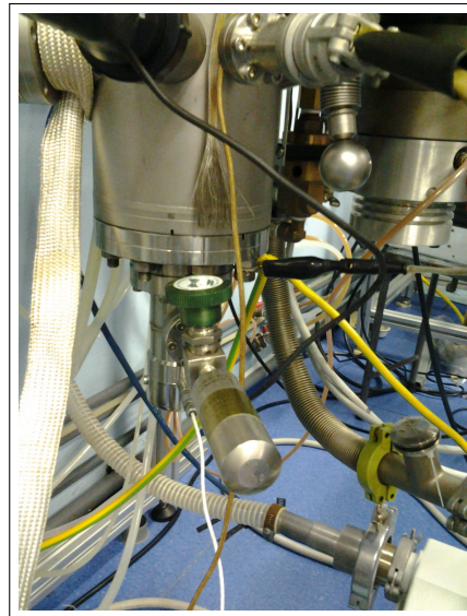
Figure 50: Ar gun for IBAD technique. Picture of the Ar ion gun recently mounted on the e-beam evaporator present at I.N.Ri.M.. The Ar gun is used for IBAD-EBPVD processes.
