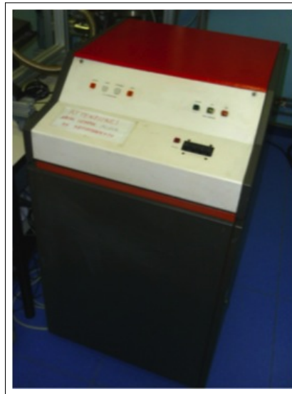
Figure 46: High Voltage generator for e-beam deposition. Picture of the High Voltage generator present at I.N.Ri.M.: the generator can receive an input voltage ranging from -9 V and 0 V and provides an output voltage of 10 kV, used to accelerate the electron beam before it reaches the target material to be evaporated.
