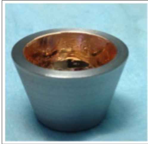
Figure 63: Mo crucible for EBPVD of Cu thin films. Picture of the crucible used for the deposition of Cu thin films: Cu, shaped in small pellets, is put inside the crucible after a careful cleaning process.
