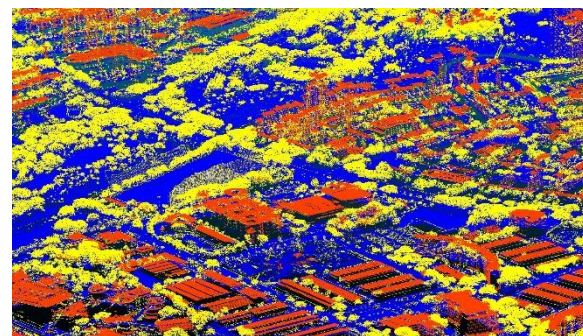
Fig. 7 – ALS data is pre-classified, here vegetation is seen in yellow, buildings in orange and the ground in blue.
