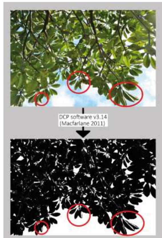
6 Fig. 3. The DCP software is not able to accurately separate foliage and sky pixels accurately when zenith images are taken in full sun conditions due to the reflection of light off some of the leaves.
