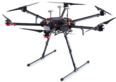
Fig. 6. The flying platform for oblique photography.
