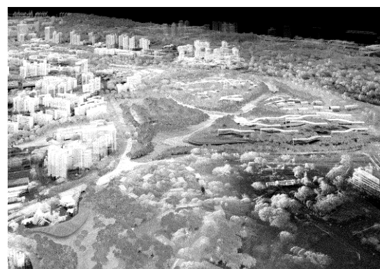
Fig. 4. Bird-view perspective of a landscape architectural design proposal on the Rail Corridor near Queenstown. The visualization is entirely based on a 3-dimensional point-cloud model. Students: Nabila Larasati Pranoto and Melissa Li Ping.
