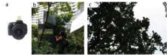
Fig. 1. The process of acquiring zenith images: (a) A DSLR camera mounted with a multi-axis spirit level was used to take zenith photographs of tree crowns; (b) Images taken of individual trees were taken when spirit bubble was levelled and the camera was pointing at the zenith angle; (c) An example of a zenith image. Images taken in urban areas will invariably include some urban features within the image, which need to be removed before analysis.
