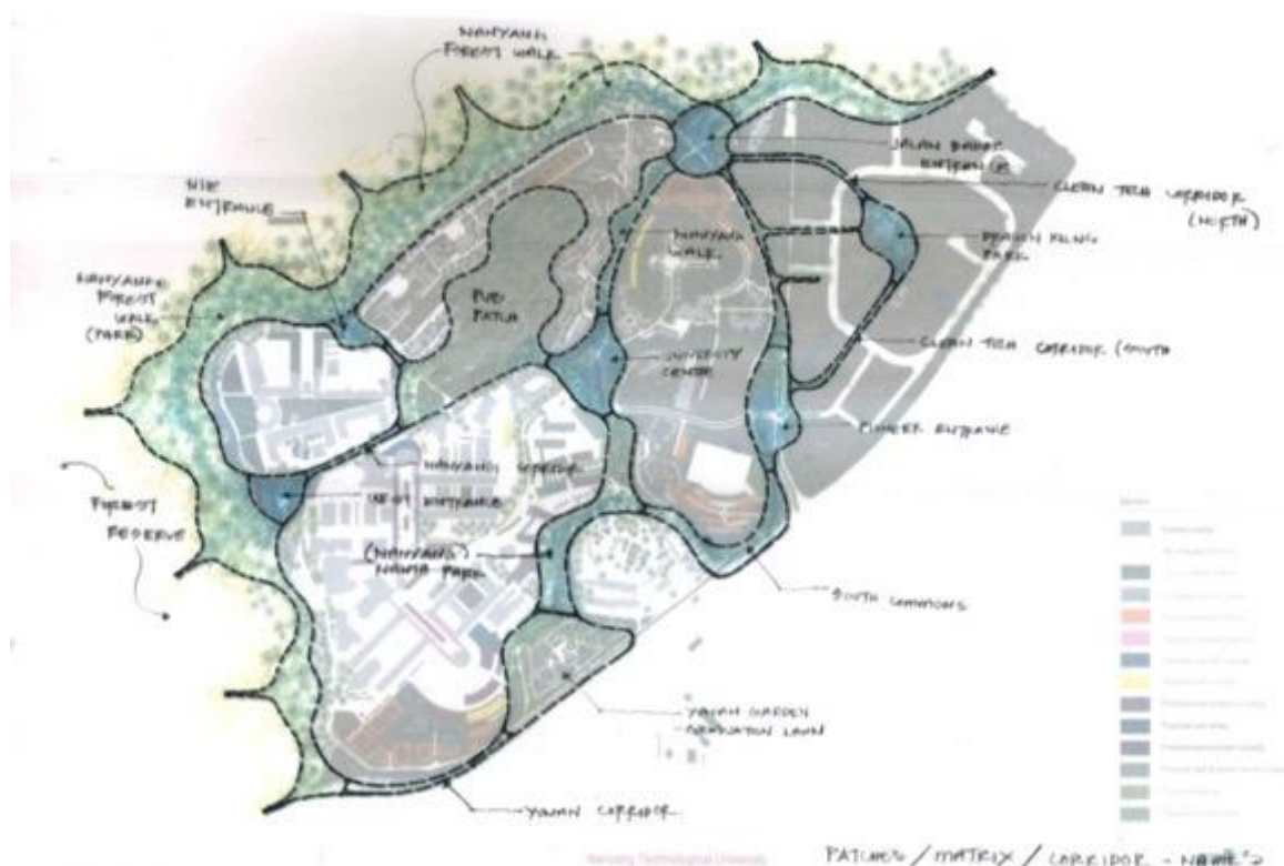
Fig. 2. Landscape Masterplan framework based on patches, corridors, and matrix theory. The corridors allow unimpeded flora and fauna movement between patches.
