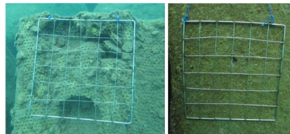
A 30 × 30 cm 2 quadrat used to monitor the fauna and flora on the ECONcrete®Antifers – left, and on the Standard Antifers – right.
