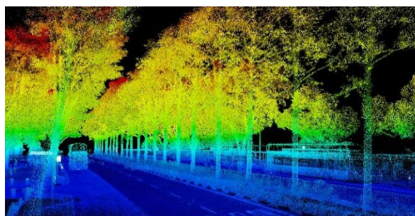
Fig. 8 – MLS data of every road in Singapore is available and as a result every tree planted along the roadside has already been scanned.
