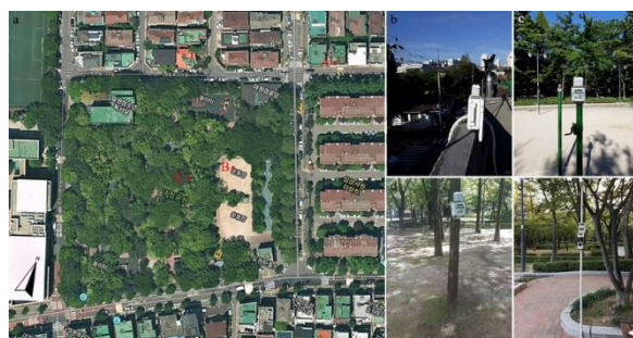
Fig. 1. Selected site for in-situ measurements: a aerial view of the Deacheong Park; b sampling point A; c sampling point B; d sampling point C; e mobile measurement: a GPS and 3 TR-72wf sensors attached to the metal pole at 0.1, 1.5 and 2 m above the ground.
