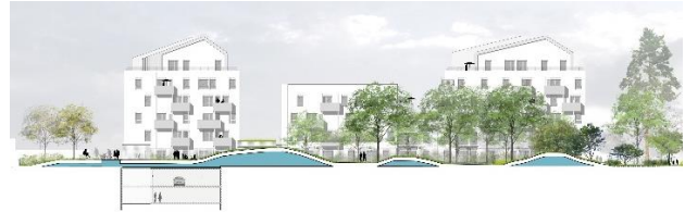
Fig 9 : Kept on site contaminated soil : under landscaped shoulders © Plan b architectes
