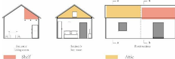
Fig. 6. The self-organized house structure which provides extra space for safe storage during the flood.
