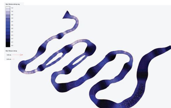
Fig.7 The flow model shows velocities up to 1 meter/sec
