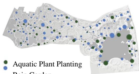
Fig. 6. Planning of Rainwater Purification System
