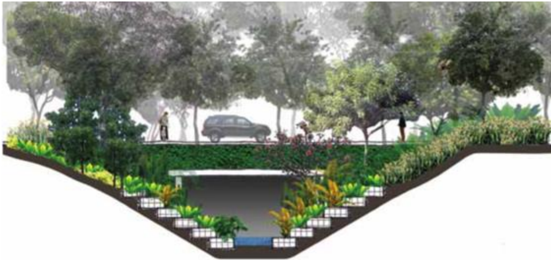
Fig. 4. Section of a Habitat Corridor underneath a Roadway. This is an example of how habitat corridor can be part of the infrastructure for the campus while at the same time utilise as a safe passing corridor for small animals to move from one habitat to another.
