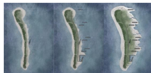
Fig. 5. Growth of an island using the concept of Building by Nature. © Maria Potamiali
