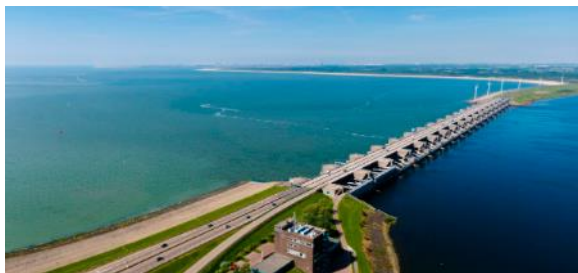
Fig. 2. Haringvlietdam, river water (on the right of the dam) can flow into the sea. The Netherlands. © maritimnieuws, RWS
