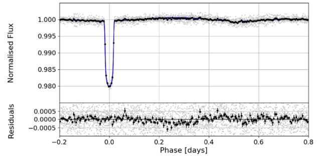
**Figure 3.** Phase folded light curve and the best-fitting transit model of EPIC 219654213. Grey points are the measurements, black circles the binned data. The continuous line represents the best-fitting model. Residuals to the fit are shown in the lower panel.
