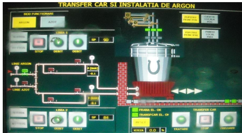
Figure 2. Online control of the bottom stirring
