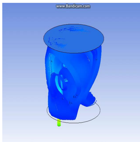
Figure 5. Bottom stirring simulation with ANSYS
