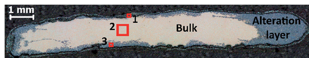
Fig. 2 Section of a late Celtic drachm attributed to the Veneti’s tribe (coin coming from a private collection). A clear alteration layer can be seen on the coin surface.
