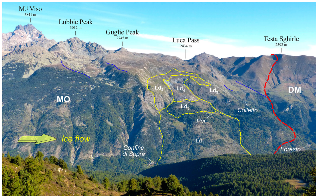
Figure 2. Panoramic view of the left side of the Varaita Valley. Red dashed line: tectonic contact between the Monviso meta-ophiolite Complex (MO) and the Dora-Maira Unit (DM). Yellow dashed lines: boundaries of the Pui-Orgiera landslide and related sectors (Ld 1 –Ld 4 ). Blue lines: lateral moraine ridges related to the Last Glacial Maximum. Photo taken from Sampeyre Pass (2283 m a.s.l.), view looking N (Long. 7°07'09", Lat. 44°33'04").
