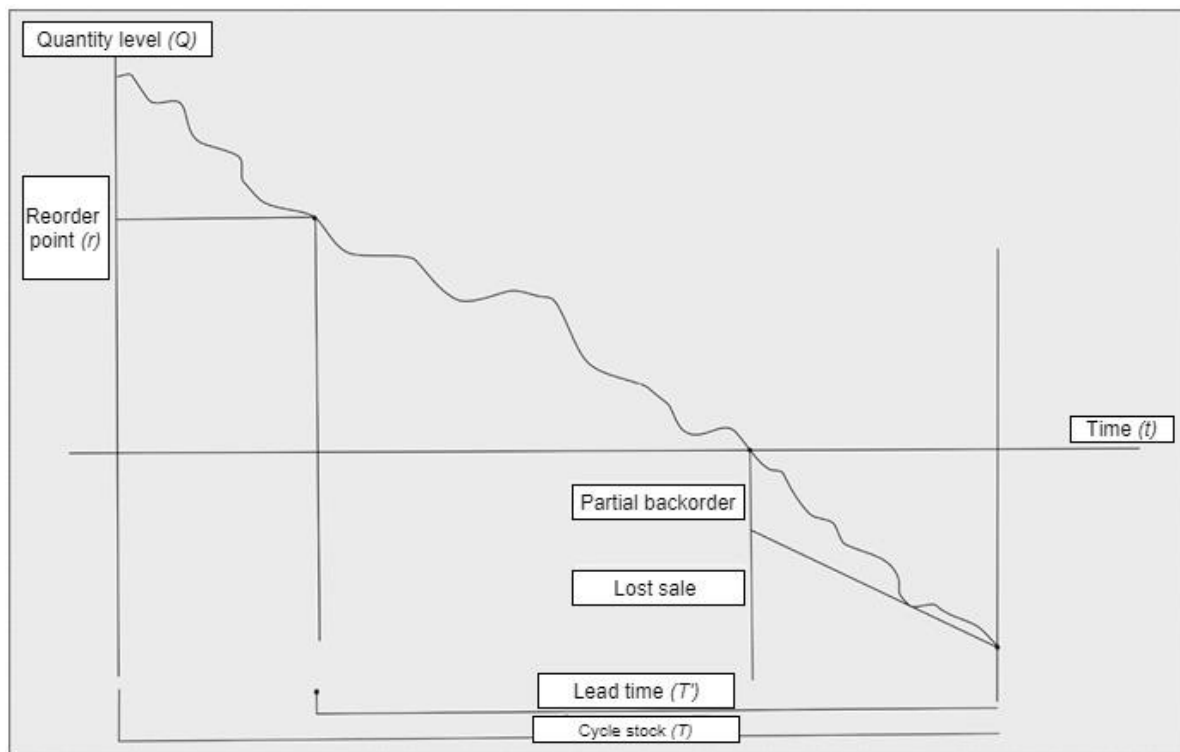
Fig 1. Continuous review inventory control system with partial backorder and lost sale
