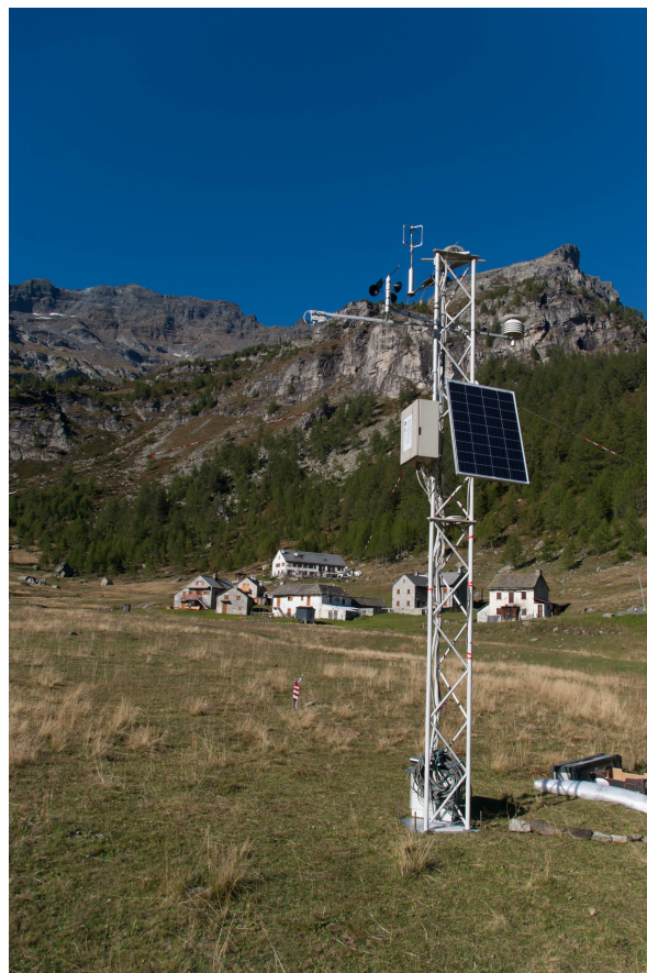
Figure 2. The 5 m tall station mast, with the ultrasonic anemometer and radiometer on the top. The snow-meter, wind vane, cup anemometer and thermometer are on the lateral arms and the barometer is behind the photovoltaic panel. The Cornù hamlet is in the background.
