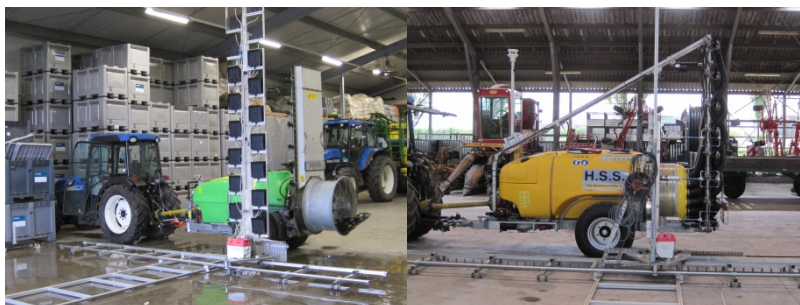
Figure 1. 3-D liquid distribution setup (left) and air-flow distribution setup (right)
