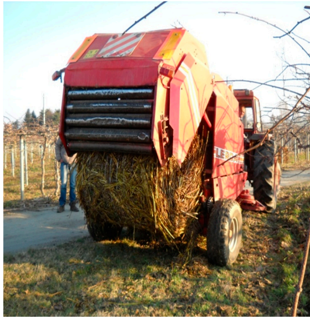
Figure 1. The agricultural round baler used to make bales.
