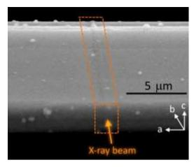
Figure 3. Scanning electron micrograph detail of the  $YBa_2Cu_3O_{7-\delta}$  crystal region irradiated with X-rays (sample B). The nanobeam is aligned along the b-axis and scanned in the a-c plane to expose the volume highlighted in orange.
