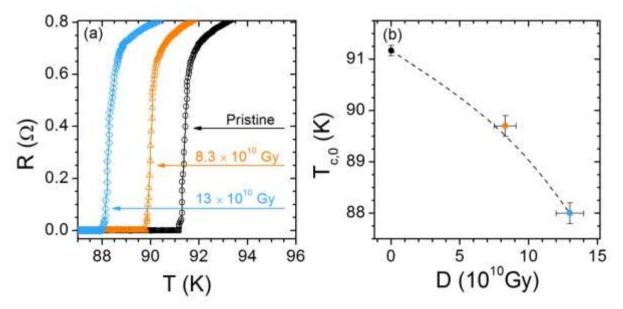
Figure 4. (a) Shift of the resistance transition measured, with a four-probe configuration, in sample B for pristine conditions (black circles) and after the first (orange triangles) and the second (light blue diamond) dose. (b) Critical temperature  $T_{c,0}$  vs absorbed dose as determined from panel (a).
