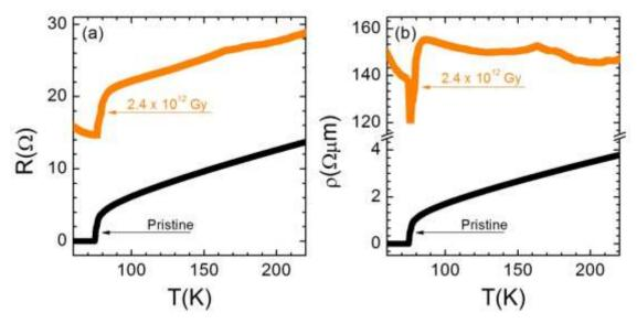
Figure 2. (a) Comparison of the electrical resistance versus temperature behavior, measured for sample A with the four-probe configuration, between the pristine state (black points) and after an X-ray absorbed dose of  $2.4 \times 10^{12}$  Gy (orange points). (b) The electrical resistivity of the irradiated  $YBa_2Cu_3O_{7-\delta}$  region (orange points) of sample A is compared to the one of the pristine state (black points). Both behaviors have been calculated from panel (a).
