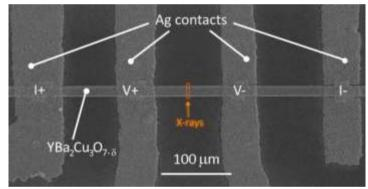
Figure 1 Scanning electron microscope (SEM) image of a typical  $YBa_2Cu_3O_{7-\delta}$  electrical device with Ag contacts in four probe configuration. In order to monitor the electrical changes induced by the X-ray irradiation we exposed the region highlighted by the orange rectangle, which is located between the voltage contacts.
