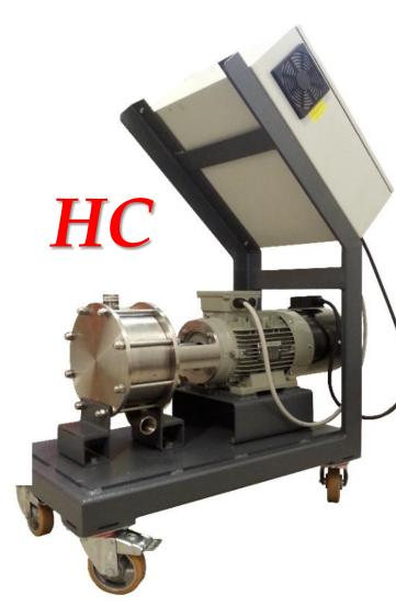
**Pilot scale reactor Rotocav**® 3000 rpm, 3 kW
