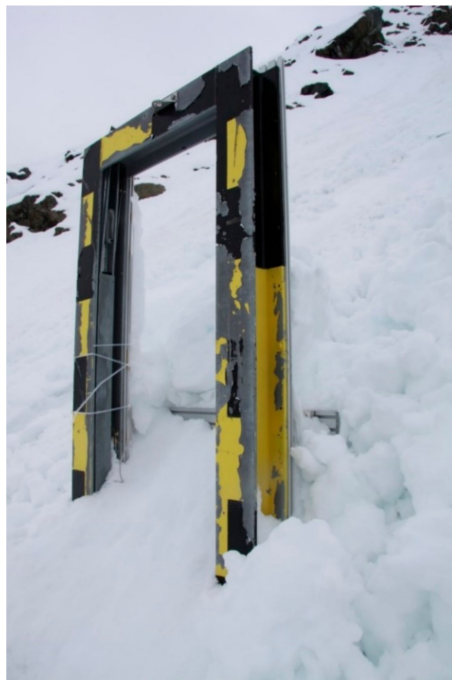
Figure 13. View of the obstacle after the event on 30 April 2014 (photo M. Maggioni on May 1). It is clearly visible that the plates are totally submerged in the snow and the large snow agglomerate against the structure.
