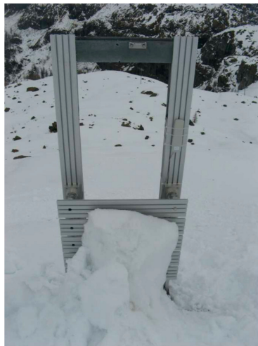
Figure 9. Deposition against the obstacle, due to the spontaneous avalanche on 17 April 2013. Photo E. Bovet on April 24.
