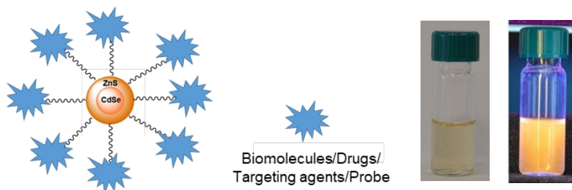
Figure 1: a) Schematic representation of conjugated QDs; b) DHLA-EDADA coated CdSe/ZnS QDs water dispersion under white and UV light.
