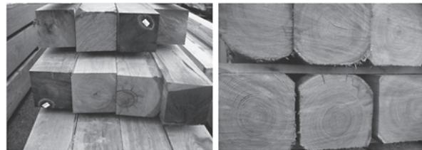
**Figure 1** Rectangular (left) and irregular (right) cross section timber for structural use is subjected to CE marking obligation since January 1<sup>st</sup> 2012
