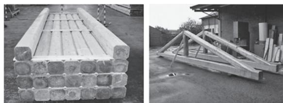
**Figure 4** “Usò fiume” spruce beams (left) and trusses realized by assembling “Usò Fiume” larch beams (right)
