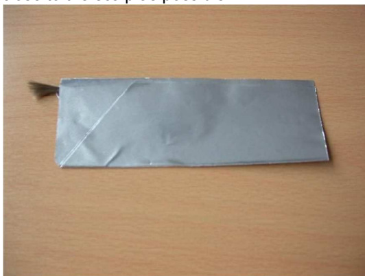
Each aluminium foil is to be folded once as shown above.
