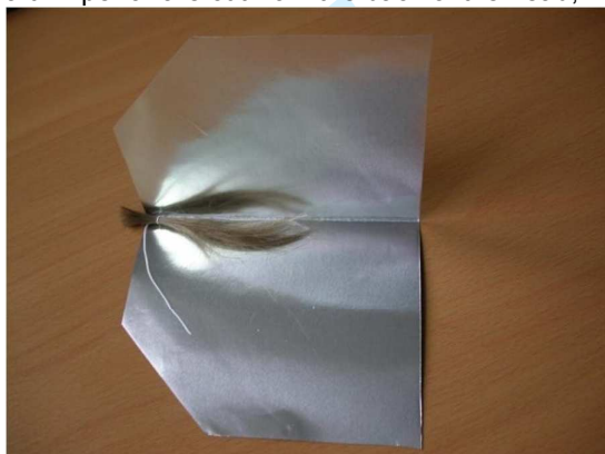
The hair lock(s) are put in separate aluminium foils provided with the root end exposed at the notched end.
