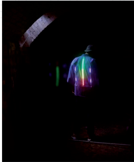
Figure 9. A running kimono. It detects one environmental variable and change the LED's light proportionally to the acquired value.
