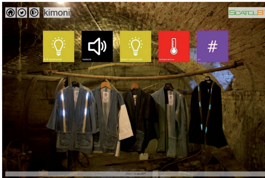
Figure 11. The smartphone app forwards the collected data to a server. In this way it's possible to check the values everywhere using a browser, not just if you are near the kimono.
