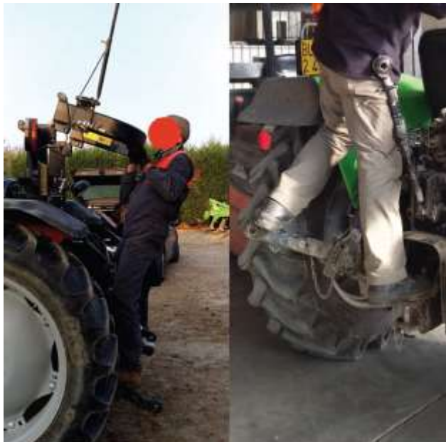
298 299 Figure 6. Examples of unbalanced and uncomfortable postures and gestures performed by 300 the operators to raise the FROPS.
