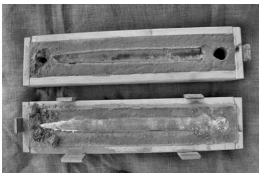
Fig. 2: Sand casting of a bronze sword. Experiment by C. Cavazzuti, L. Pellegrini, F. Scacchetti.
