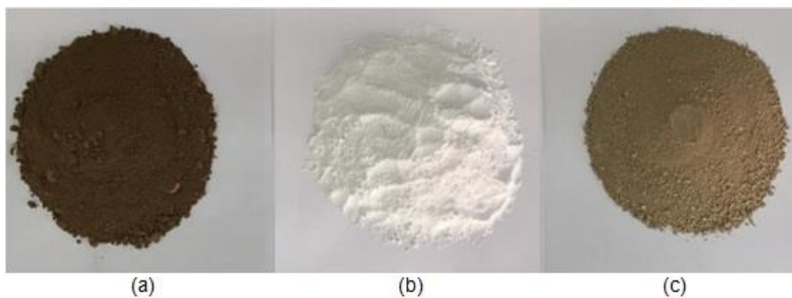
Figure 1. a – crude oil-contaminated soil; b – neutralizer; c – neutralized soil.
