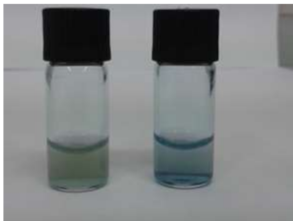
Figure S3 Functionalized TiO 2 nanoparticles before (left) and after covalent linking to BSA (right), both stained with Bradford reagent. The blue color of the suspension containing BSA-TiO 2 confirmed successful conjugation of the protein.
