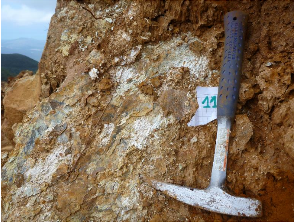
Figure 2. Fibrous-lamellar antigorite showing several degrees of alteration on the outcrop, Koniambo massif, New Caledonia (from Mission XTRATA Amiante 2012).
