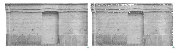
Figure 6. NIR models for dataset 2: Metashape Professional (left) and Zephyr Aerial (right).
