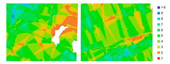
Figure 4. Number of overlapping images on the area of interest for scenarios 3 (left) and 4 (right).
