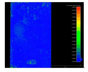
**Figure 8.** Variation between VIS and NIR Metashape Professional models for dataset 3 (Hausdorff distances shown on a scale up to 8 mm, with 0.5 mm scalar field intervals).
