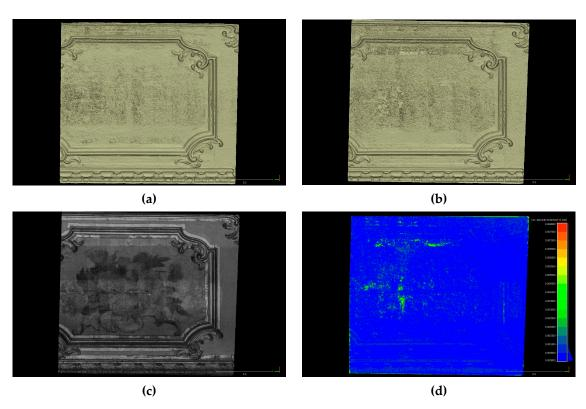
**Figure 9.** Dataset 3 meshes produced with Metashape Professional, (a) untextured VIS mesh, (b) untextured NIR mesh, (c) vertices textured NIR mesh, (d) distances between NIR and VIS meshes.
