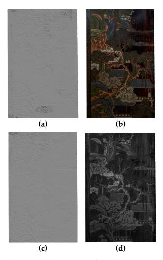
**Figure 7.** Dataset 3 meshes produced with Metashape Professional, (a) untextured VIS mesh, (b) textured VIS mesh, (c) untextured NIR mesh, (d) textured NIR mesh.
