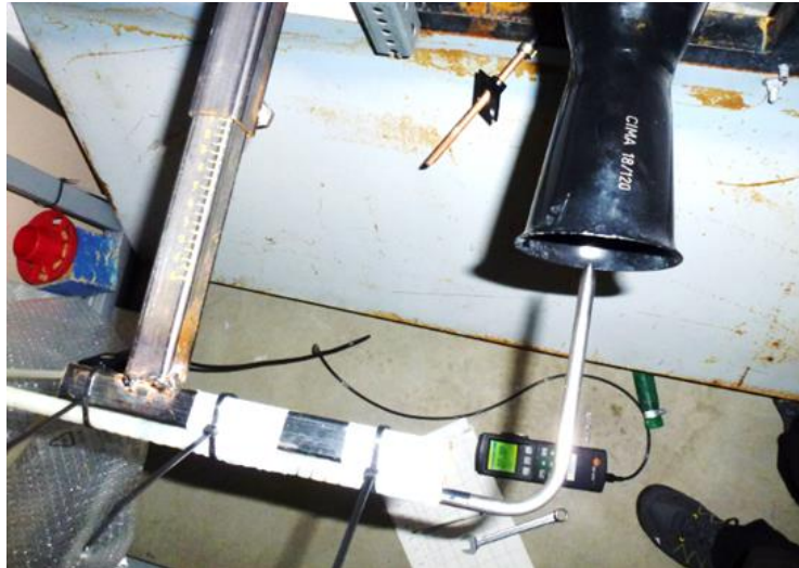
Figure 5. Implement for measuring the air speed in the centre of the air spout.
