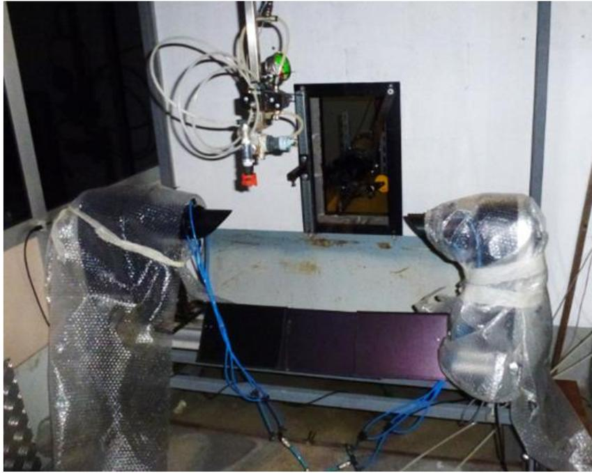
Figure 6. Malvern SprayTec® droplet size analyser.
