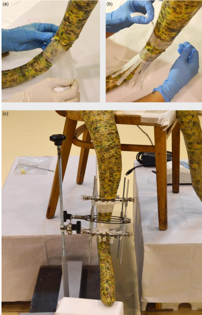
Figure 19.6 Set-up of the traction system: Placing of the two Japanese paper protecting strips on the artwork (a); positioning of the forty PLP5 tie rods, half on the upper strips likewise on the lower (b); positioning of the artwork inside the external traction system and anchoring of the tie rods to the movable rings with bulldog clips (c).
