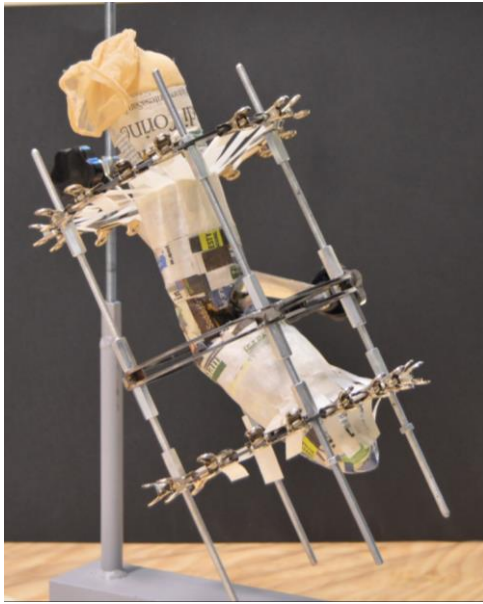
Figure 19.4 System d) before lengthening. System d) is characterized by the use of two Japanese paper sheets as a protecting layer and 10 mm wide by 130 mm long 70% polypropylene-30% cellulose pulp (PLP5) tie rods.
