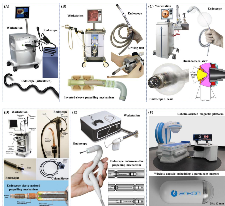
Figure 3. Examples of certified robotic flexible colonoscopes (commercially-available or certified but no longer on the market): (A) NeoGuide Endoscopy System (NeoGuide Endoscopy System Inc., Los Gatos, CA USA) [88]; (B) Invendoscope™ SC40 (Invendo Medical GmbH, Weinheim, Germany) [88]; (C) Aer-O-Scope System (GI View Ltd., Ramat Gan, Israel) [81]; (D) ColonoSight (Stryker GI Ltd., Haifa, Israel) [82]; (E) Endotics System (ERA Endoscopy Srl, Pisa, Italy) (Courtesy of ERA Endoscopy Srl) [88]; (F) NaviCam® (Ankon Technologies Co, Ltd. Wuhan, Shanghai, China) [87].
