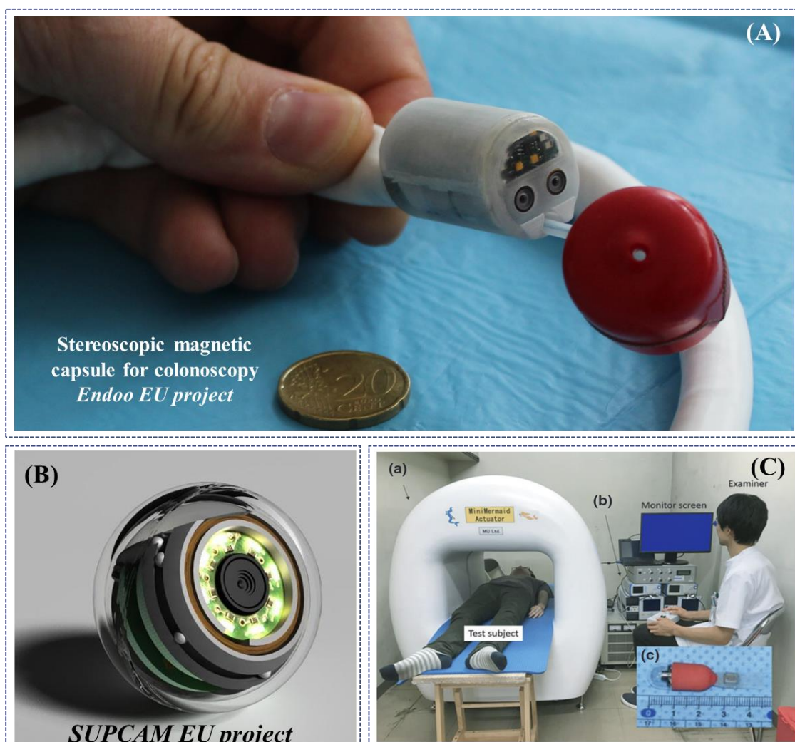
Figure 6. Examples of research-oriented innovative robotic colonoscopes and devices with magnetic or electromagnetic actuations: (A) Endoo EU project capsule (Courtesy of the Endoo consortium); (B) SUPCAM EU project spherical magnetic capsule for colonoscopy (Courtesy of Dr. Alessandro Tozzi); (C) modified PillCam™ SB2 with a silicone fin for magnetic locomotion through external electromagnetic fields, developed by Nouda et al. [128].
