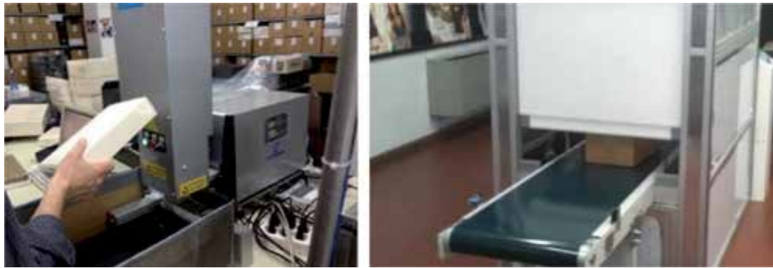
Figure 3. RFId reading post, Box label printing and application. Source: Oscalito.
