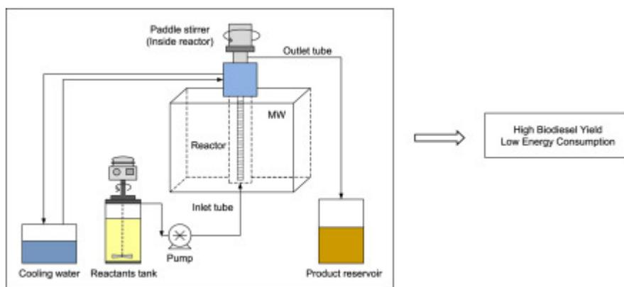
**Figure 1.** Scheme of the MW equipment used [11].
