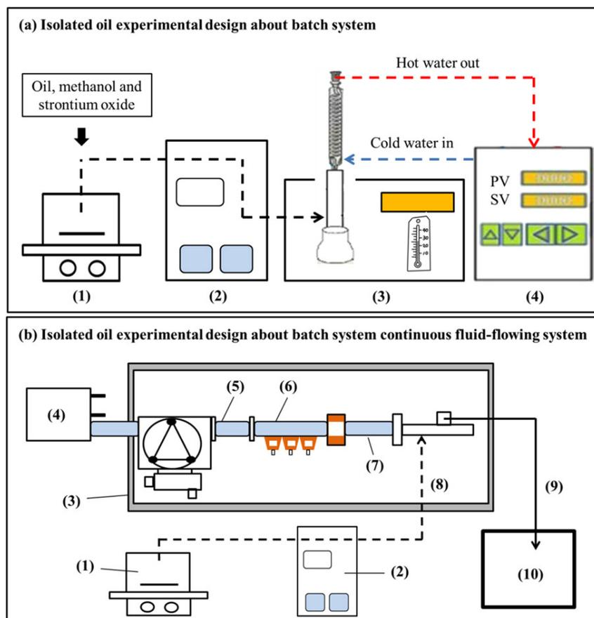
**Figure 10.** Scheme of batch (above) and continuous (below) MW systems for biodiesel synthesis. 1 to 4 in (a) correspond to magnetic stirrer, peristaltic pump, MW and cooling system. 1 to 10 in (b) denote mean stirrer, pump, MW, magnetron head, MW power, three-stub tuner, MW chamber, pipe for input, pipe for output and tank, respectively [54]
